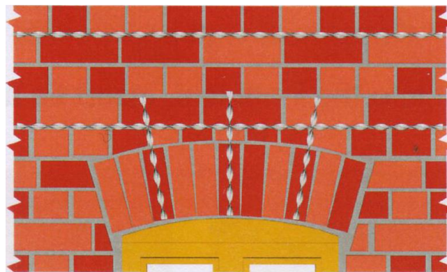
Repair and reinforcement of damaged wall lintels
