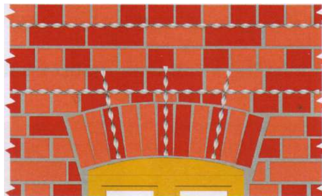
Repair and reinforcement of damaged wall lintels
